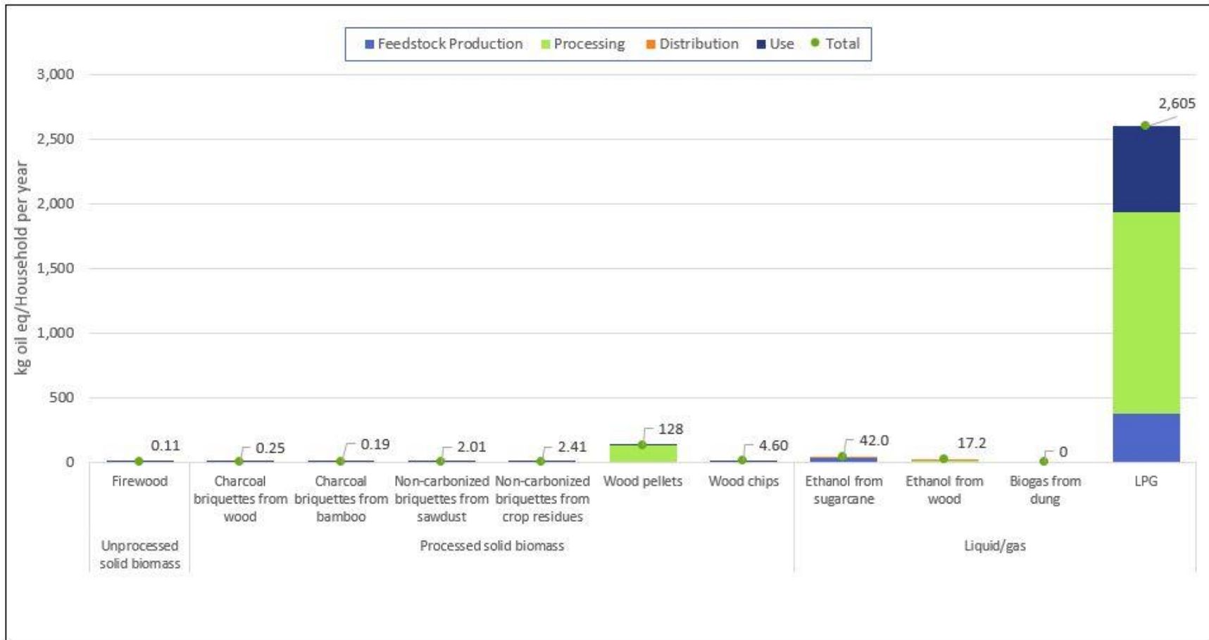
Figure A-55. Fossil Fuel Depletion Impacts (kg oil eq) for Cooking Fuel Types (Nigeria) To produce, distribute and use cooking fuels by a single household per year
